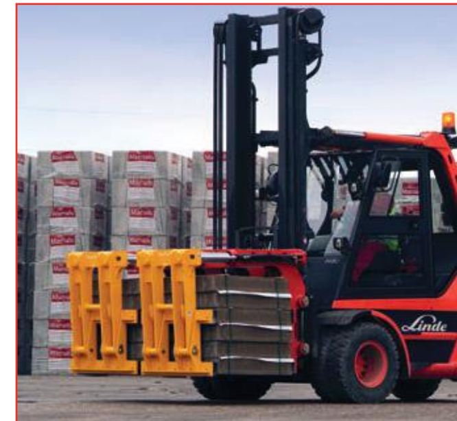
TK53 Twin Overhead Block Clamp Fixed non moving rear arm
