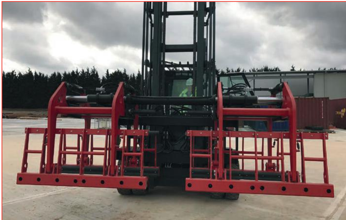
WR500T Twin Overhead Block Clamp (for 4 pack handling)
